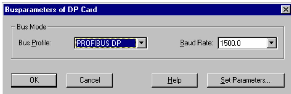
If a message indicating a baud rate error appears, repeat the procedure in subsection 2.8.5, reducing the baud rate to match the rate of the slowest DP device. Then return to the beginning of the procedure in this subsection (3.4)
