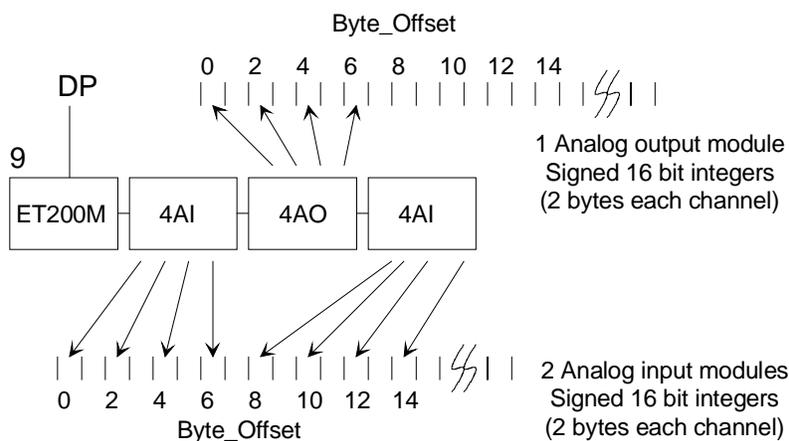
**Figure 3–7 Byte\_Offset for Typical Input and Output Block**
