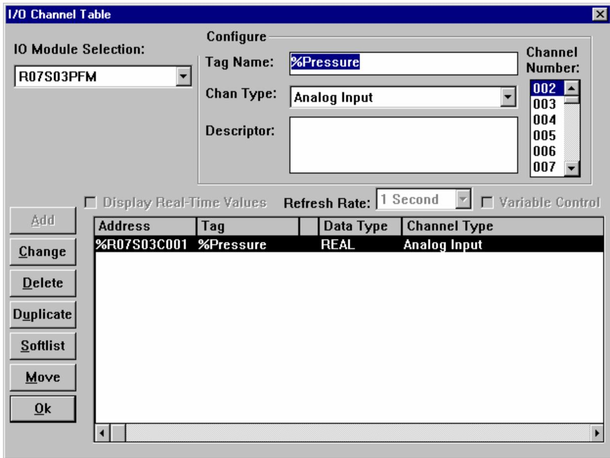
10. For each PROFIBUS field I/O point in turn, assign a channel, selecting among the available channel types:
