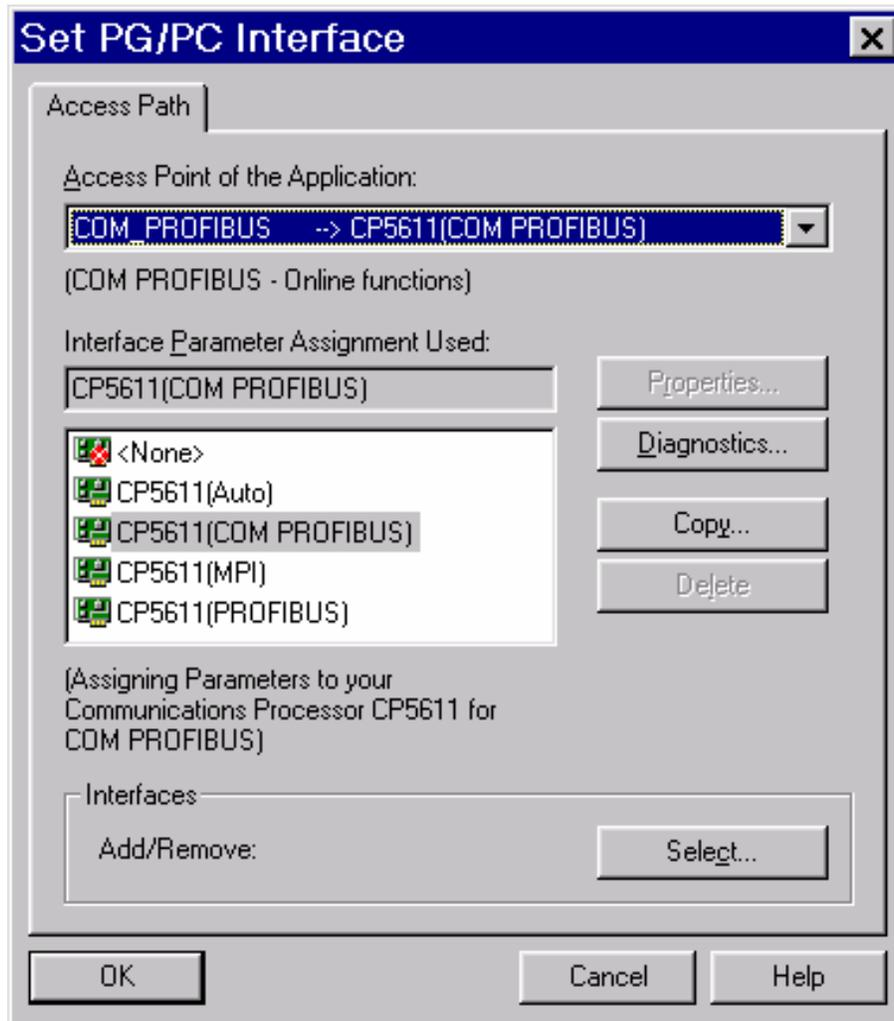
**Figure 2–4 Access Point for COM PROFIBUS**
