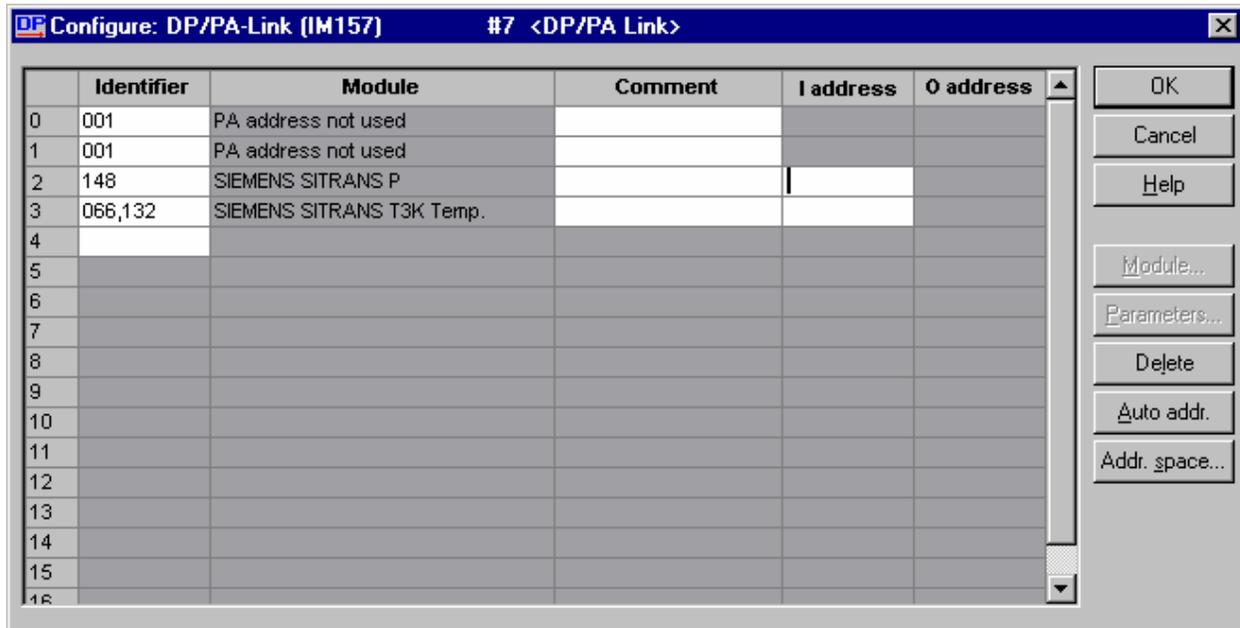
**Figure 3–3 PA Devices Occupying Positions in DP/PA Link**
