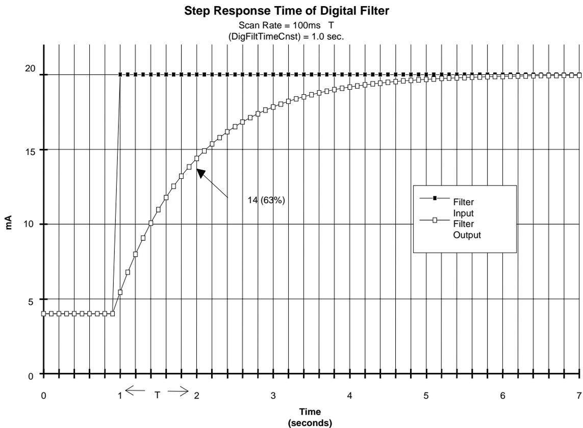
**Figure 3–15 Step Time Response of Digital Filter**
