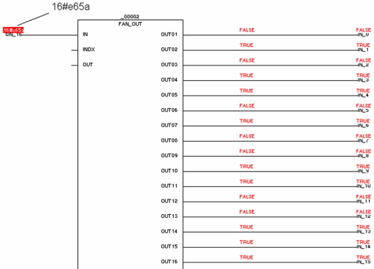
Figure 3–11 Fan-Out to 16 Bits
