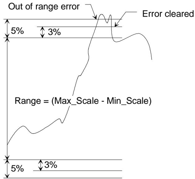
Figure 3-16 Out of Range Error and Hysteresis
