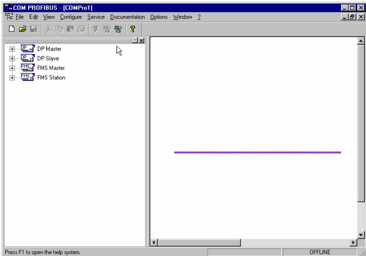
2. Populate the PROFIBUS DP network by expanding the DP Master and DP Slave lists in the left pane, also known as the “Hardware Catalog,” then dragging and dropping devices into position on the PROFIBUS DP bus, represented by the purple line. You must add a master first. Start with the PFM module.
