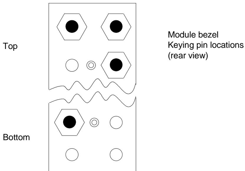
**Figure 2-3 Module Rack Mechanical Keying**
