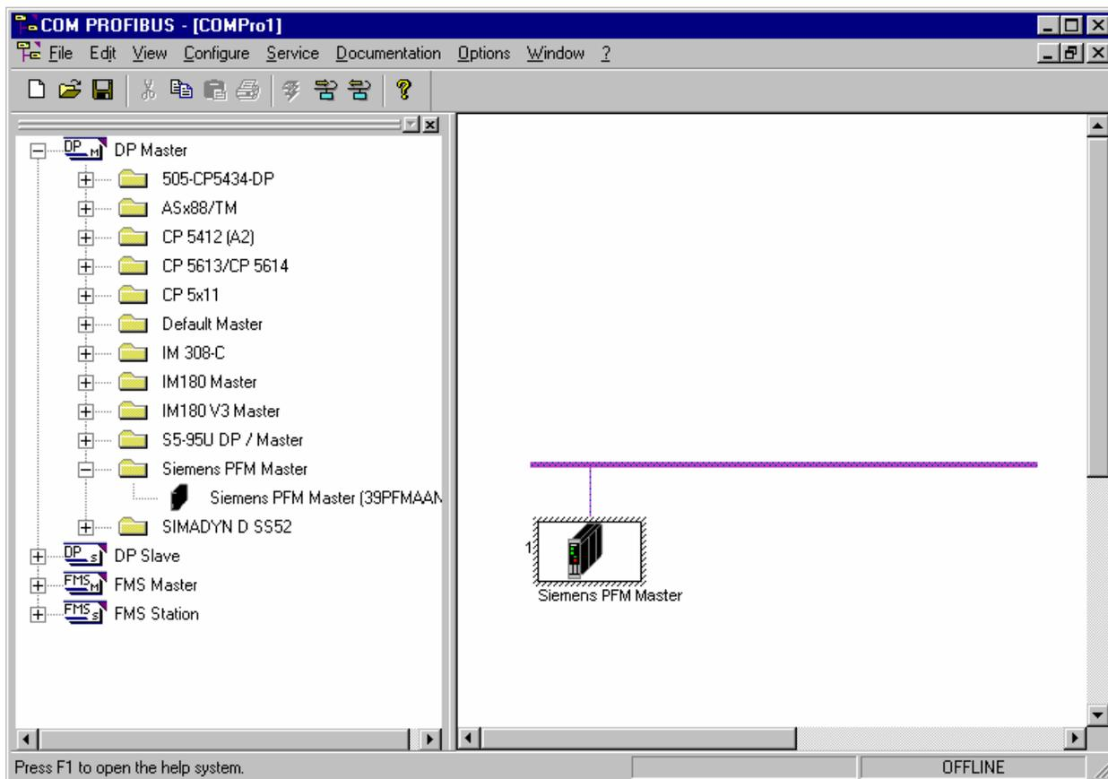
Note that the COM PROFIBUS has assigned the first available PROFIBUS address, 1, to the device. As additional devices are placed on the bus, the program increments the PROFIBUS address from the lowest available number. An address assigned automatically may be inappropriate and may require modification.
