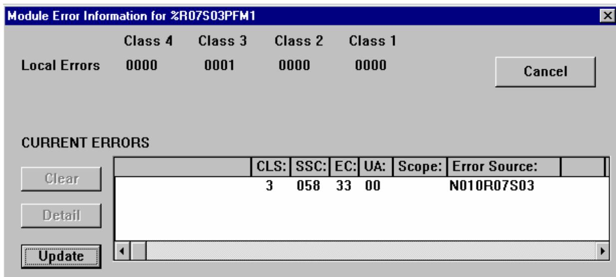
**Figure 3–6 Error Message When PFM Configuration Changes**
