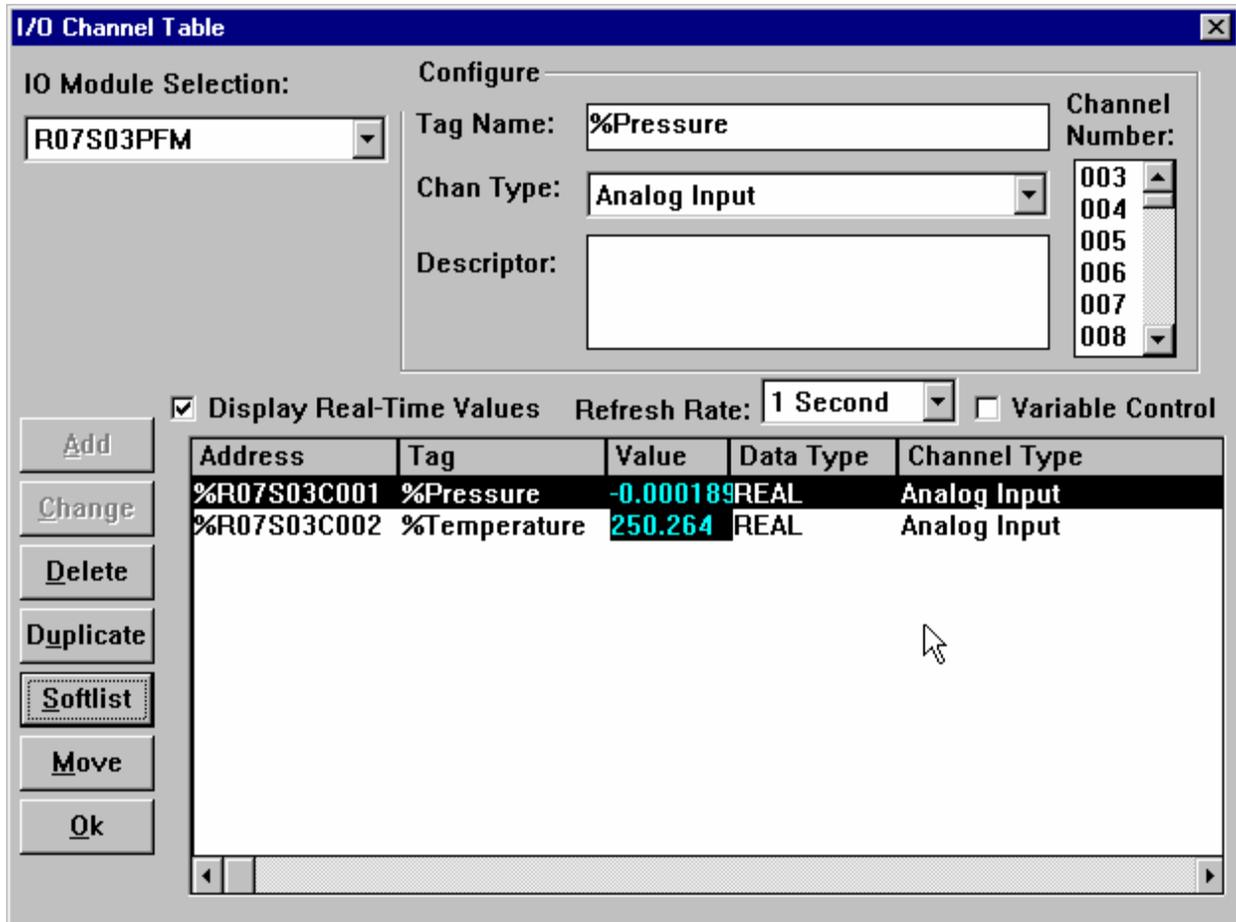
Comprehensive testing of this kind requires the services of staff who are able to force field I/O to inject values into the channels scanned by *4-mation*. Similarly, by enabling variable control on output channels, it may be possible to compare expected results with observed results.
