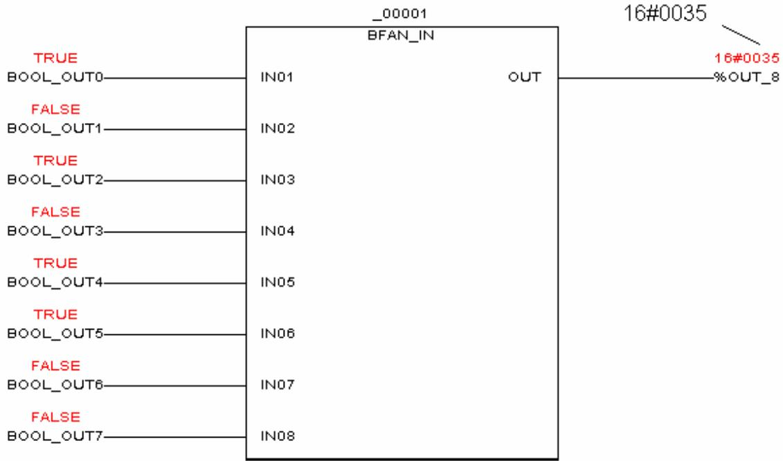
**Figure 3–14 Fan-In from 8 Bits**
