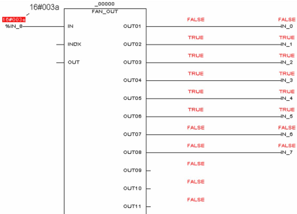
Figure 3–13 Fan-Out to 8 Bits
