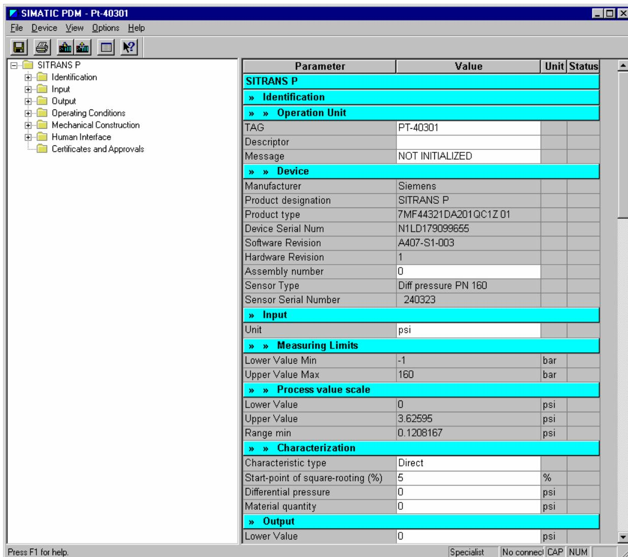
14. When you are satisfied with your choices, you can send them to the device using the menu bar selection Device > Load to Device. The program will make a connection to the device at this point if it is not already connected.
