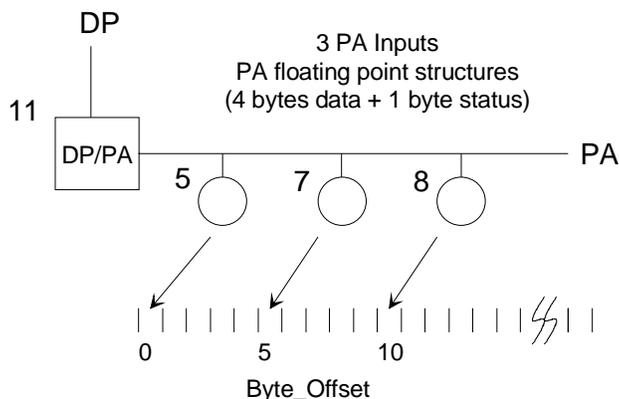
**Figure 3–8 Byte\_Offset for Typical Input String**
