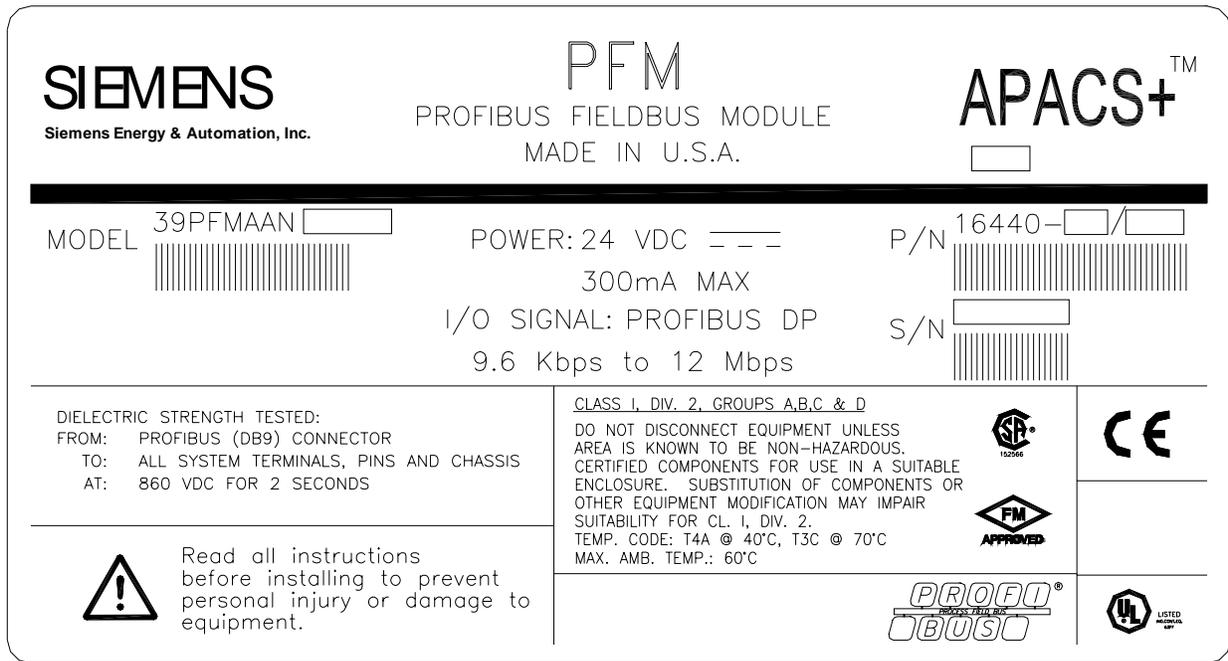
Figure 2–1 Typical PFM Module Identification Label
