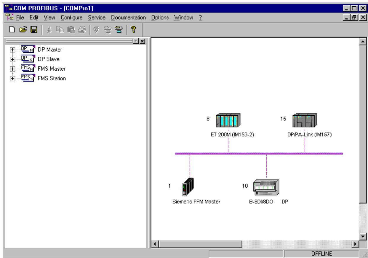
**Figure 3–1 Typical PROFIBUS DP Network with an DP/PA-Link**
