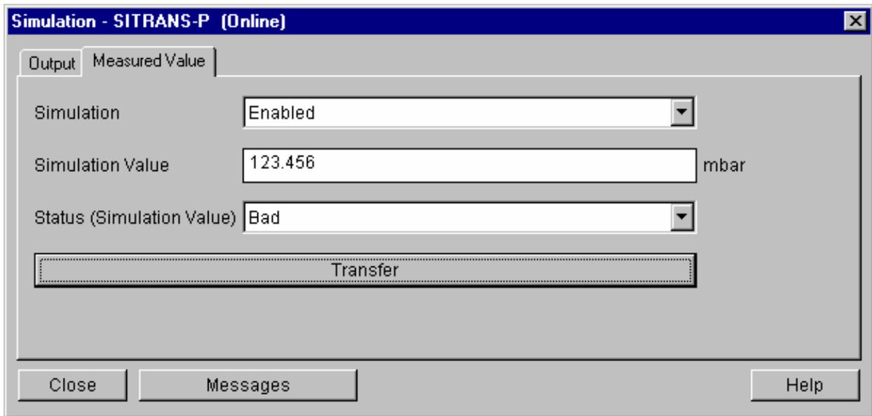
Figure 3-4 PDM Simulation Window for SITRANS-P
