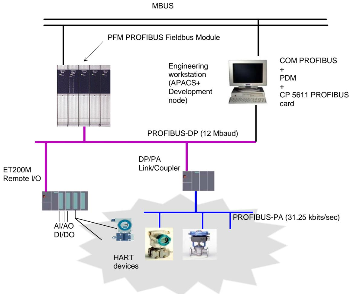
**Figure 1–1 APACS+ PROFIBUS Fieldbus Module (PFM) in a Typical Architecture**
