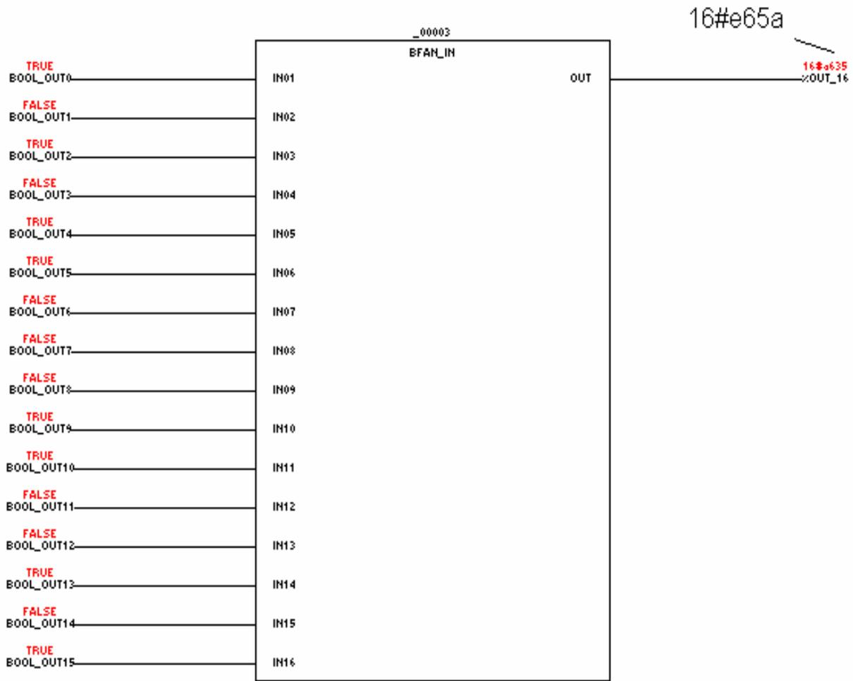
Figure 3–12 Fan-In from 16 Bits
