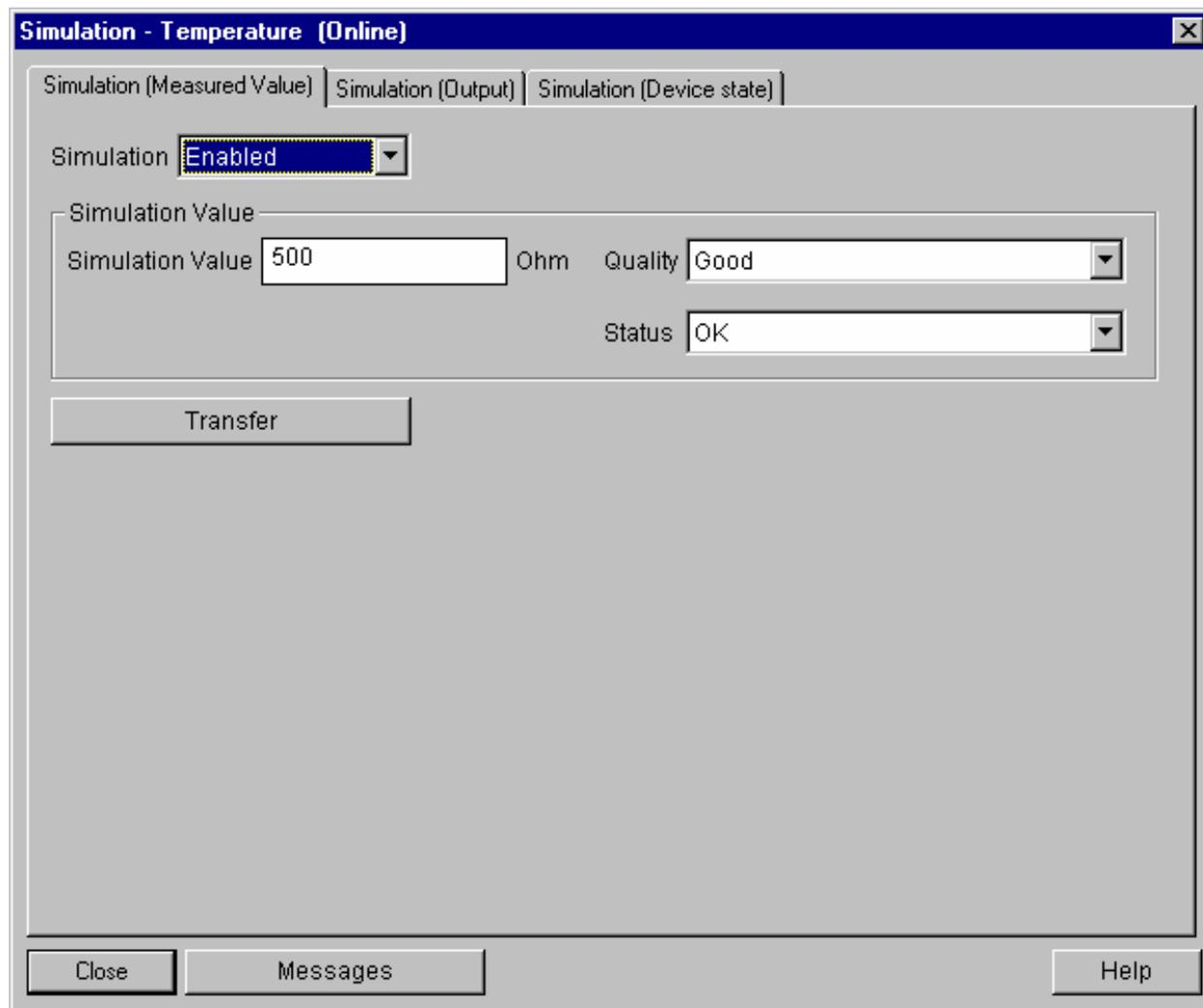
Figure 3–5 PDM Simulation Window for SITRANS-T3K
